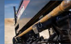
2 Add-a-pipe feature places individual pipes into loading system without lifting pipe into the top of the pipe box
