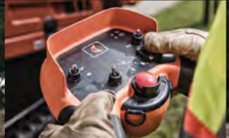
4 Optional wireless remote ground drive increases flexibility when moving the rig and allows fine-tuning of bore path placement.
