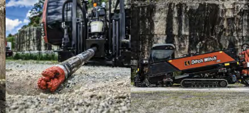
Optimized for industry-leading performance and productivity in hard rock conditions, the Ditch Witch® AT40 All Terrain directional drill is designed with an advanced version of the proven Ditch Witch All Terrain drilling system. The updated, two-pipe system offers boosted power to the bit—33 percent more torque than competitive units. Patented design enhancements increase cycle times, improve durability and allow for more adaptable steering.
